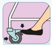
Before removing the plastic seat, secure all four castors to help prevent the chair moving away from you.
